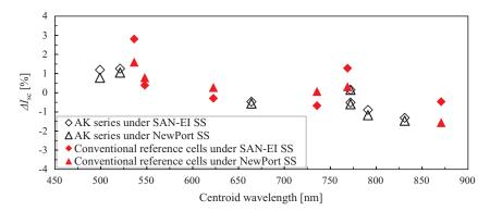
Figure 8 Difference in the short-circuit current (Δ*I*<sub>sc</sub>) between *I*<sub>cal</sub> and *I*<sub>mes</sub> calculated from equation (9) for the reference cells (Konica Minolta AK series and conventional reference cells made by other companies) under the solar simulators.
