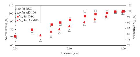
Figure 11 Changes in the solar cell efficiency (η) and open circuit voltage (V<sub>oc</sub>) determined for DSC-NIMS-2 and AK-100 upon irradiance with a solar simulator. DSC-NIMS-2, dye-sensitized solar cells-National Institute for Materials Science.
