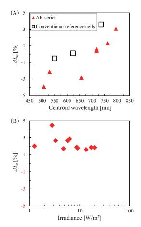
Figure 10 (A)  $\Delta I_{sc}$  determined for the reference cells under LED with an irradiance of 3.97 W/m<sup>2</sup> and (B)  $\Delta I_{sc}$  determined for nonlinear cells by changing the irradiance of LED.
