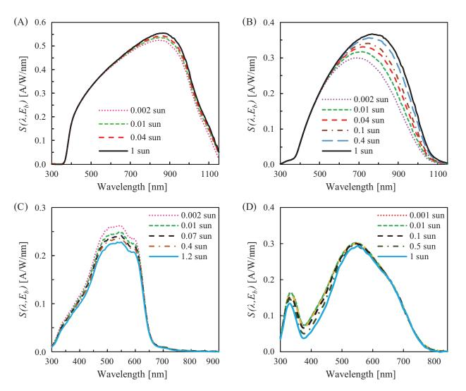
Figure 7 Spectral responsivity (*S*(λ, *E*<sub>b</sub>)) determined for two nonlinear cells (cells A and B), OPV and DSC-B: (A) Cell A, (B) Cell B, (C) OPV, (D) DSC-B. DSC, dye-sensitized solar cells; OPV, organic thin film solar cell.
