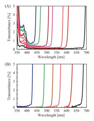
Figure 2 Transmittance level of stray light determined for: (A) a conventional spectroradiometer; and (B) the spectroradiometer equipped in this device.
