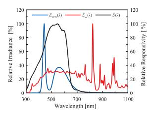
Figure 12 Relationship between the spectral responsivity of the OPV  $(S(\lambda))$  and spectral irradiance of the light sources ((E\_LED( $\lambda$ ) for LED, E\_ss( $\lambda$ ) for the San-ei Electric XES-40S (1 sun)). OPV, organic thin film solar cell.
