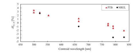
Figure 5 Difference in the short-circuit current among the calibration centers plotted against the centroid wavelength.
