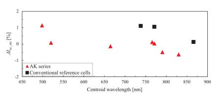
Figure 6 Difference in the short-circuit current (ΔI<sub>sc\_stc</sub>) between that determined by the PRISM SK-1150 unit and that determined at a calibration center for linear cells under STC plotted against the centroid wavelength of the spectral responsivity (*W*<sub>c</sub>). PRISM, Programmable Reference cell system for Irradiance adjustment by Spectral Measurement; SK-1150, Spectral responsivity unit; STC, standard test conditions.
