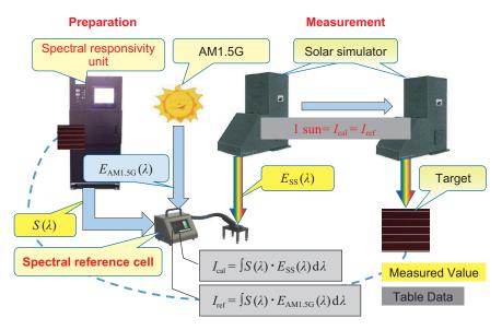
Figure 1 Schematic diagram of the PRISM system. PRISM, Programmable Reference cell system for Irradiance adjustment by Spectral Measurement.
