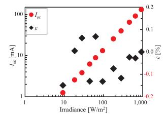
Figure 3 Short-circuit current ( $l_{sc}$ ) and linearity error ( $\epsilon$ ) of SRC-1100 plotted against the irradiance. SRC, spectral reference cell.
