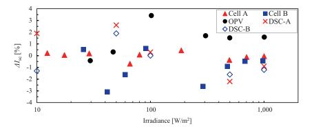
Figure 9 Δ*I*<sub>sc</sub> determined for two nonlinear cells (cells A and B), OPV, DSC-A and DSC-B under the solar simulator. OPV, organic thin film solar cell; DSC, dye-sensitized solar cells.
